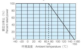
在环境温度70 $^{\circ}$ 以上使用时,应按照左图负荷特性曲线,减小额定功率。 For resistors operated at an ambient temperature of 70 $^{\circ}$ Cor above, a power rating shall be derated in accordance with derating curve on the left.
